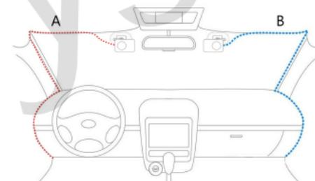
Step 4: Connect the cable with the Dashcam, Turn on the ignition to test the installation.
