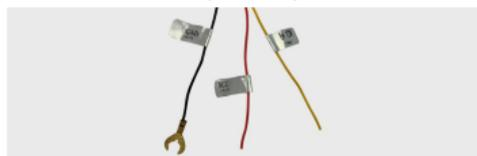
a RED wire marked ACC, which connected with Fuse Box ACC, can make auto turn on&off when the vehicle is on&off.
