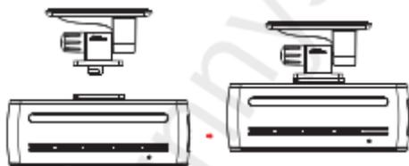
3. Remove the protective film from the back of the bracket, attach the adhesive side of the bracket on the windshield where it has an unobstructed view of the road but does not interfere with the driver's view. As shown below.
