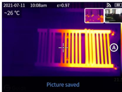
Press the "Shutter" button in the real-time preview interface, "Photo saved" appears and a 2s thumbnail is displayed in the top right corner.
