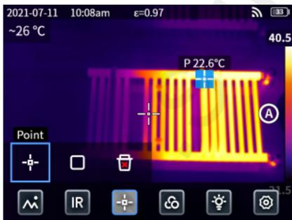
Click **☰** to open the hidden status bar, and then click **☰** to add a point analysis object and click **□** to add a rectangular analysis object. Long press the rectangular analysis object to set the maximum temperature, the minimum temperature, the average temperature, the area and the center of the object and to delete the object.
