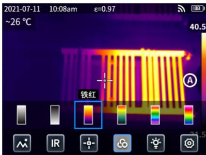
点击...按钮,打开隐藏的状态栏,再点击
