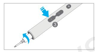
2. Press 3, tighten the screws.
